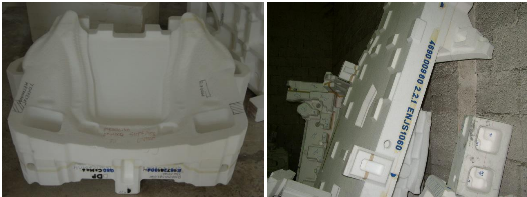
Material removed in different patterns in order to prevent extra-large zones. Usual practice agreed by many patterns
