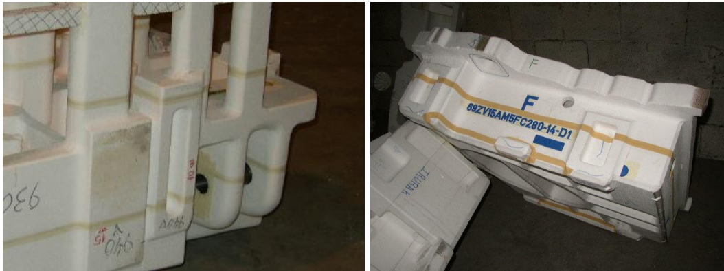
Material removed in different patterns in order to prevent extra-large zones. Usual practice agreed by many patterns
