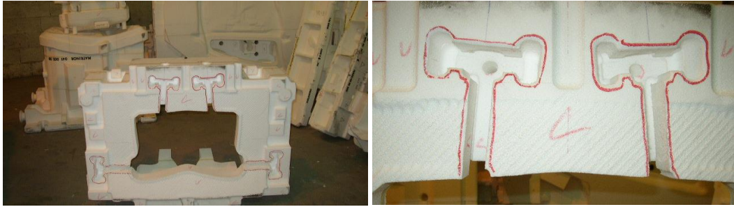
Pattern with four deep grooves for lift housing and through hole inside for lift guide
