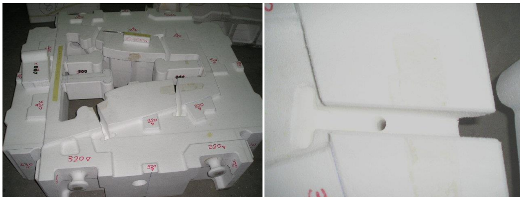
Mortise with machining ridges and hole for the lift cylinder to pass through
