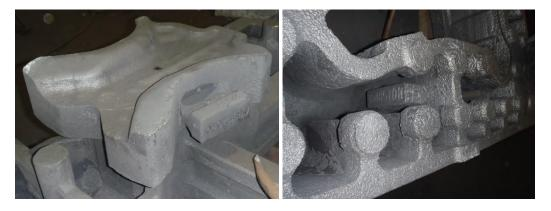
Samples stuck to copies or profiles should not be placed, as this would cause hot spots that may lead to contraction defects (shrinkages).
