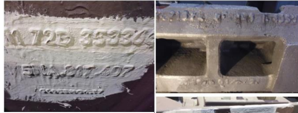
Defects originating from using hollow letters.
