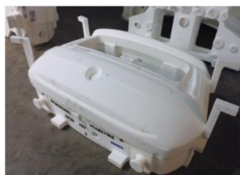
ERRONEOUS LEG CONCEPT EXCESSIVE PROTRUSION
